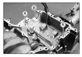
• Install the drive shaft and output shaft into the upper crankcase half.
