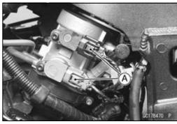
• Loosen the holder clamp Allen bolts [A].
