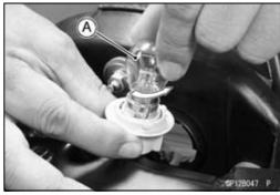
Insert a new bulb [A] by aligning its upper pin [B] with the upper groove [C] in the socket, and turn the bulb clockwise.
