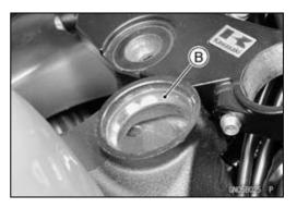
Remove the lower inner race [A] (with its grease seal [B]) which is pressed onto the steering stem with a suitable commercially available bearing puller or chisel [C].
