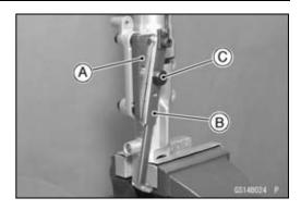
OCompress the outer tube holding the front fork by using the lever [A] of the spring compressor to insert the stopper [B] into the hole [C] with the lever hole aligned with the holder hole.
