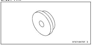
Lead Wire - Voltage Regulator Adapter: 57001-1448
