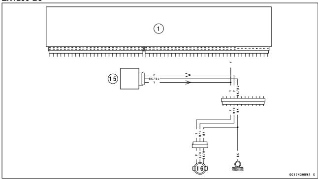
ECU [1] Meter Assembly [15] Speed Sensor [16]
