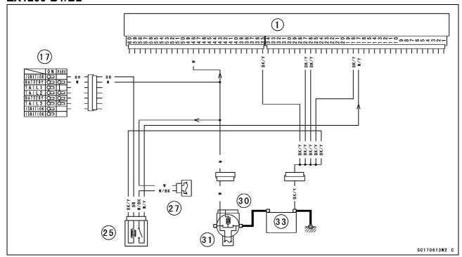
→: Current ECU [1] Ignition Switch [17] ECU Main Relay [25] ECU Main Fuse 15 A [27] Starter Relay [30] Main Fuse 30 A [31] Battery [33]
