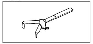
Valve Seat Cutter, 55° -  $\phi$ 35: 57001-1247
