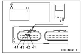
★If the output voltage is out of the standard, remove the left lower inner cover, and check the output voltage at the injector connector [B] using a digital meter [A] and needle adapter set [C] (when the lead is open, the output voltage is 0 V).
