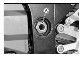
Unscrew the swingarm pivot shaft nut [A].
