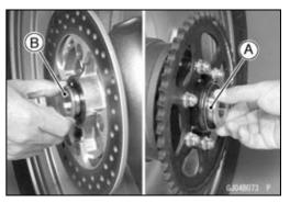
Olf the coupling is removed from the rear wheel, apply the grease as shown.
