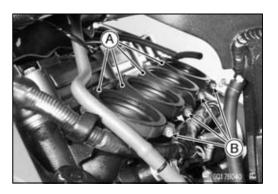
• Be sure the fuel hose [A] are clamped securely to prevent leaks.
