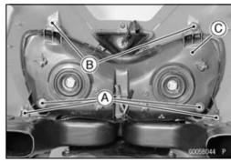
Remove: Screws [A] City Light Assembly [B]
