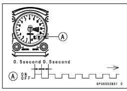
Olf there is any problem in the registration, the FI indicator light [A] blinks to display the collation error. Immobilizer Amplifier Failure
