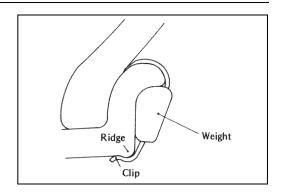
• When required total weight exceeds 20 g (0.71 oz), install balance weight at both sides of rim flange as shown.
