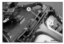
• Lift the front portion of the fuel tank [A] and support it with the supporting rod [B].
