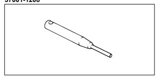
Rotor Puller, M16/M18/M20/M22 × 1.5: 57001-1216
