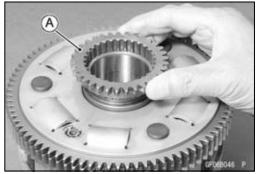
• Align the teeth of the clutch housing gears by the gear setting [A].
