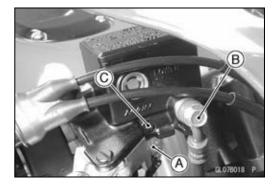
• Unscrew the clamp bolts [A], and take off the master cylinder as an assembly with the reservoir, brake lever, and brake switch installed.
