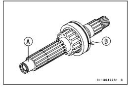
• Aligne the bushing-oil holes [B] with the shaft-oil holes to install the gear bushings [A].
