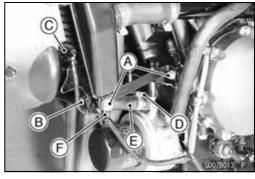
Right Horn Bolt [A] Right Horn [B]
