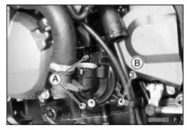
Remove the water pump cover [A] by inserting the screw driver to the pry point [B] on the water pump housing [C].
