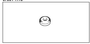
Valve Seat Cutter, 30° -  $\phi$ 30: 57001-1120
