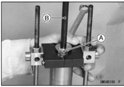
• Install the rebound damping adjuster rod [A].
