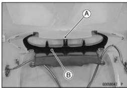
• Remove the screw [A] to take off the plate [B] and turn signal light.
