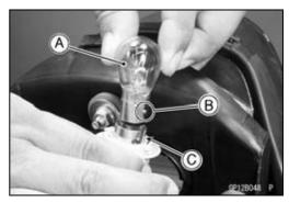
• Insert the socket by aligning its projection [A] with the upper groove [B], and turn it clockwise.
