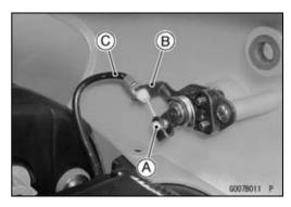
Remove: Screws [A] Seat Lock [B]
