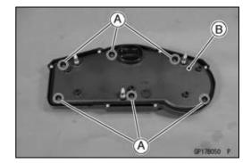
• Separate the meter assembly [A] and meter covers [B].
