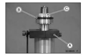
Holding the top plug [A] with a wrench, tighten the piston rod nut [B] against the top plug.
