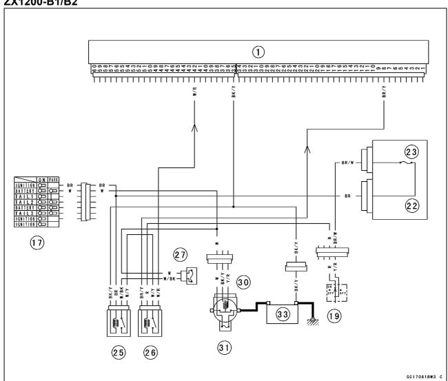
$\rightarrow$ : Signal ECU [1] Ignition Switch [17] Engine Stop Switch [19] Junction Box [22] Ignition Fuse 10 A [23] ECU Main Relay [25] Fuel Pump Relay [26]
