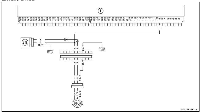
ECU [1] Meter Assembly [39] Speed Sensor [40]
