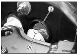
Tail/Brake Light Lens Assembly Replacement
