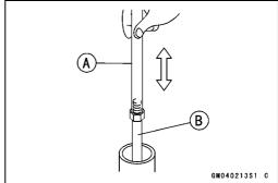
Oil Level (fully compressed, without spring) Standard: 93 ±2 mm (3.66 ±0.08 in.)
