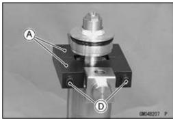
• Insert the holder bar [A] into the axle hole of the front fork [B].
