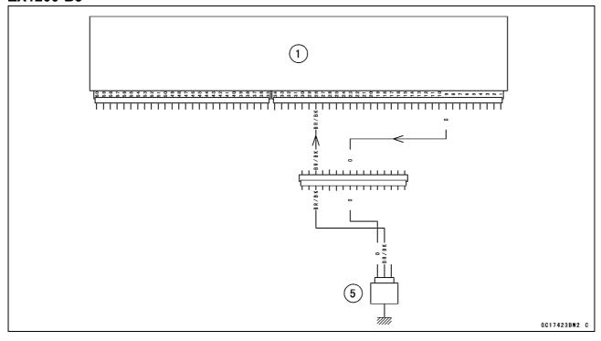
→: Signal ECU [1] Water Temperature Sensor [5]
