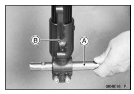
• Insert the compression shaft [A] and install the nut.
