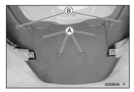
• Take off the screw [A] to remove the air inlet [B].
