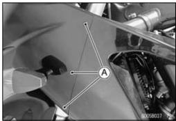
• Loosen the left and right air inlet duct clamp screws [A].
