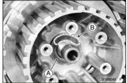
• Replace the clutch hub nut with a new one.
