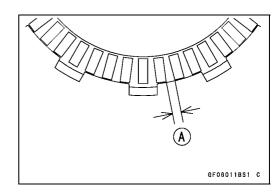
Olnstall the last friction plate [A] fitting the tangs in the grooves in the housing as shown.
