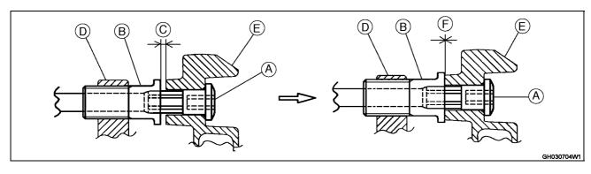
Hold the upper and lower engine mounting bolts with an Allen wrench, and tighten the nuts [A] with specified torque.
