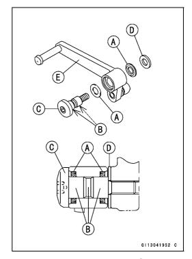
Install the shift pedal [A] so that the center of the shift pedal front end [B] is aligned with the center line [C] of the shift rod [D] by loosening the front and rear locknuts [E], and turning the rod.
