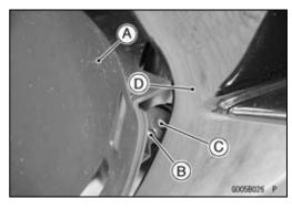
OPull out the lower fairings [A] to clear the its grommets [B] from the projections [C] of the upper inner fairings [D].
