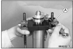
• Holding the piston rod nut with a wrench [A], remove the top plug [B] from the piston rod.
