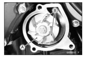
Water Pump Housing Disassembly
