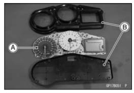
Remove the screws [A] to separate the inner and outer cover of the upper cover.
