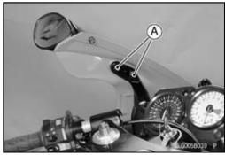
Remove the projections [A] on the left and right upper inner fairings [B] from the grommets [C] on the left and right lower fairings [D] pulling out the lower portion inward of the upper inner fairings.
