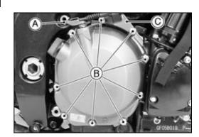
• Turn the release lever [B] toward the rear [C] as shown, and remove the clutch cover [A].
