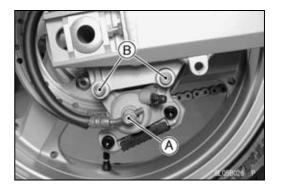
Remove the pistons, dust seals and fluid seals as same as front caliper disassembly.
