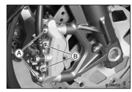
Remove: Pad Pin [A] Pad Spring [B]
