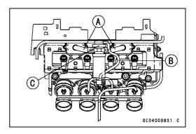
Vacuum Switch Valve Installation (ZX1200-B1/B2)
