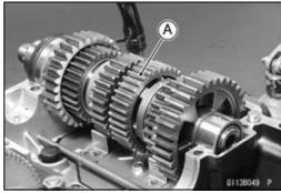
OThe bearing set pins and rings must match properly with the holes or grooves in the bearing outer races. When they are properly matched, there is no clearance between the crankcase and the bearing outer races [A].
