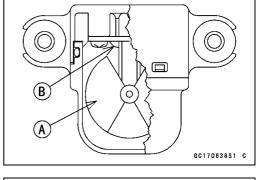
When the motorcycle is down, the ignition switch is left ON. If the starter button is pushed, the electric starter turns but the engine doesn't start. To start the engine again, raise the motorcycle, turn the ignition switch OFF, and then ON. When the ignition switch is turned ON, current flows through the latch-up circuit and the transistor in the circuit is turned ON to unlock the latch-up circuit.
