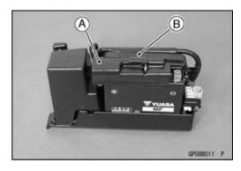
Remove: Positive (+) Cable [A] Battery [B]
