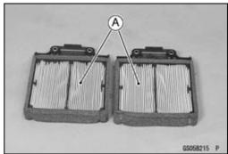
Install the elements [A] with the mark side (FRONT) facing front.
