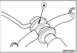
Vacuum Switch Valve Test (ZX1200-B1/B2)
