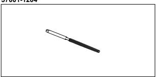
Valve Seat Cutter Holder,  $\phi$ 5: 57001-1208
