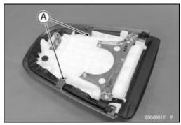
• Remove the front bracket portions [A] from the projection [B] of the seat.
