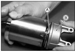
• Remove the terminal locknut [A] and terminal bolt [B], and then remove the brush with the brush plate [C] from the left-hand end cover.
