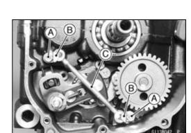
Remove the shift shaft assembly [A] while pulling the shift mechanism arm [B] to the direction of the arrow.
