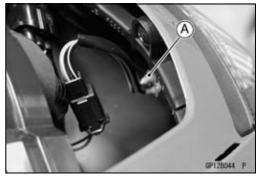
• Pull the bulb [A] out of the socket.
