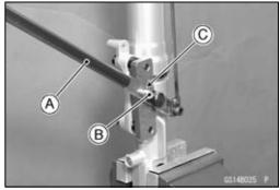
OHolding the piston rod nut [A], remove top plug [B] from the push rod with wrenches.
